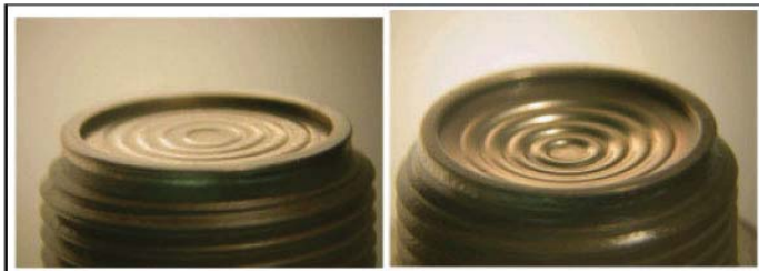
Figure 2. Photographs of the upper end of a normal Druck pressure sensor (left) and one with a deformed titanium diaphragm, indicative of the microleak problem (right).
