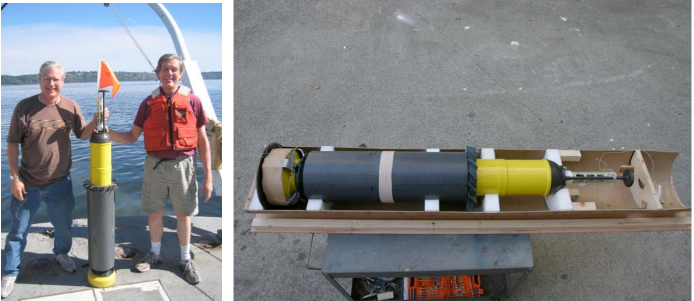
Figure 2: Left panel shows the EM-APEX and its developers, senior engineers Jim Carlson (L) and John Dunlap (R), during Puget Sound testing. Only the grey PVC shell with electrodes and the small turbine blades for instrument rotation are added to the exterior of Webb Research Corporation's APEX float. Right panel shows the EM-APEX in the bottom half of the air-launch container. The air-launch container is completed with the addition of the other half for the cardboard cylinder and a parachute. The container is held together with nylon straps that are released by salt blocks that dissolve in about an hour after being immersed in seawater.
