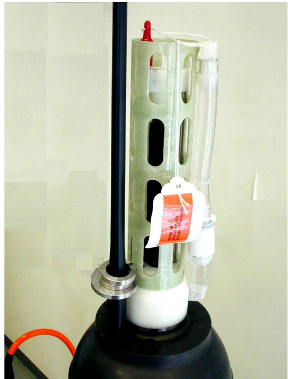
Photo2. Weights for rough ballasting (rings put on the antenna).
