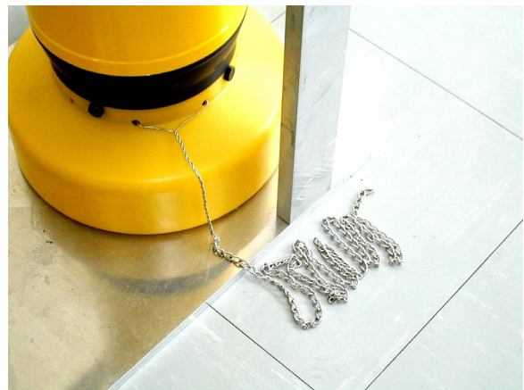
Photo3. Chain with attachment to the float.
