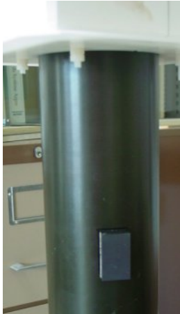
ON/OFF Magnet Position (Float is Powered ON if magnet removed)
