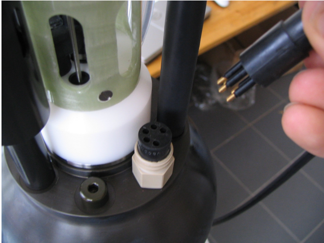
Figure 10.2: Connection of terminal connector to the float.
